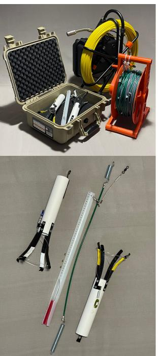
The Extractor is a state-of-the-art "well rescue" tool specifically designed for the **retrieval of lost objects from environmental testing wells, bore holes and drilling sites.** When used in the field, its rapid and precise extraction capabilities minimize costly delays and the need for expensive well redrilling.
